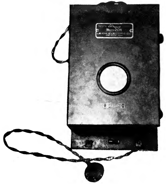
FIG. 8 An A battery charger of the vibrating type
